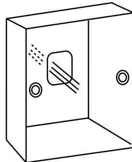
3.Fix back cover to the holder. After that, connect communication wire to CON1 port of wired controller. Finally put the front cover of wired controller to back cover to complete the installation.
